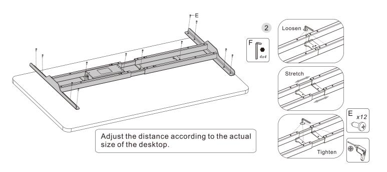
Use method 2 in Step 6 to install the desktop, when the desk frame is stretched to more than 1720mm.
